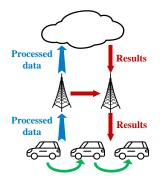
Fig. 1. Data processing model in an edge-based solution.
